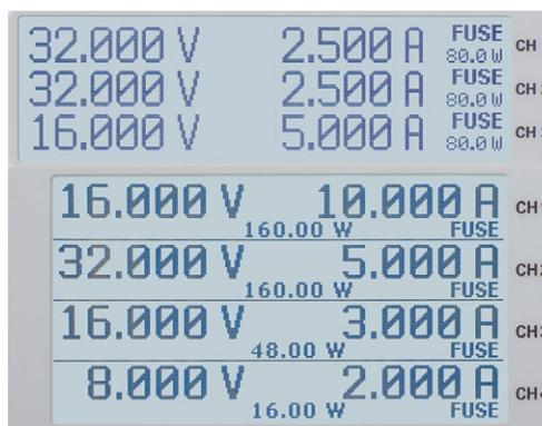
Fig. 4.7: HMP2030 / HMP4040 Fuse appearance in the display
