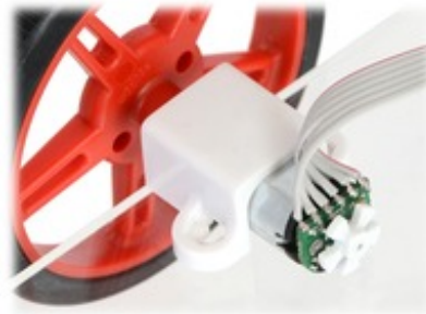
Example of an installed micro metal gearmotor reflective optical encoder.
