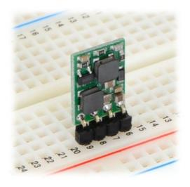
This regulator is also available with a fixed 5 V output or a fixed 9 V output.
