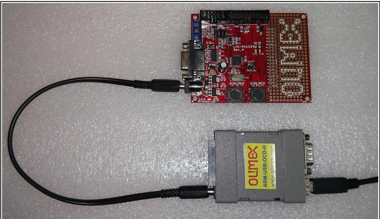
ARM-USB-OCD-H powering LPC-P11C24 (via the PWR_OUT jack).
