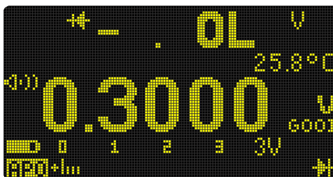
Figure 2-24 Auto-diode display (GOOD status)
