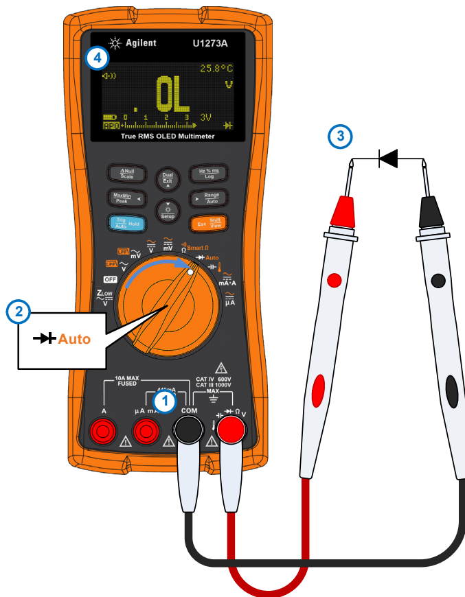
Figure 2-23 Testing a reverse-bias diode
