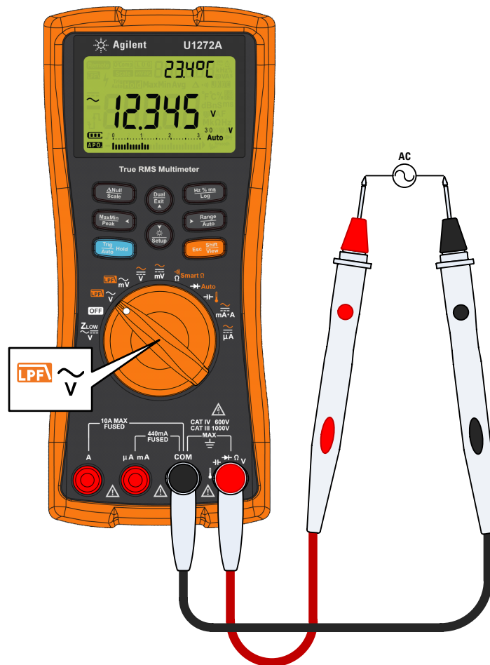
Figure 2-2 Measuring AC voltage
