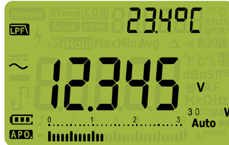
Figure 2-3 AC voltage with LPF display
