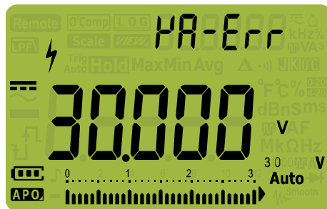
Figure 1-3 Input warning display
