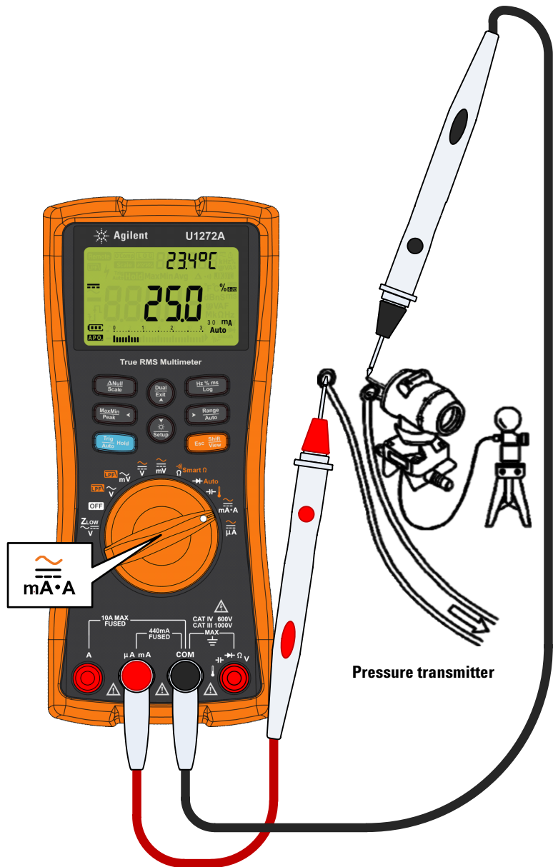
Figure 2-35 Measuring DC current using the 4-20 mA % scale
