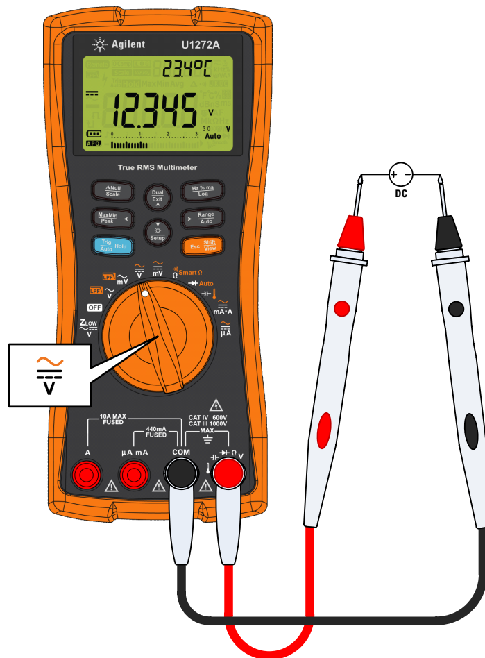
Figure 2-5 Measuring DC voltage
