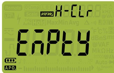
Figure 3-10 Empty view display
