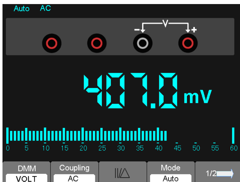
Figure 7-7 AC voltage Measurement
