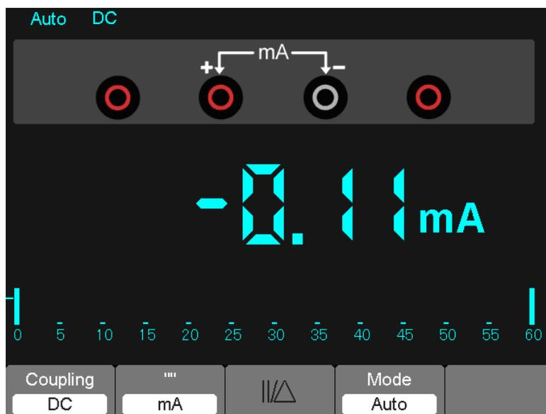
Figure 7-8 DC current Measurement for 600 Measurement
