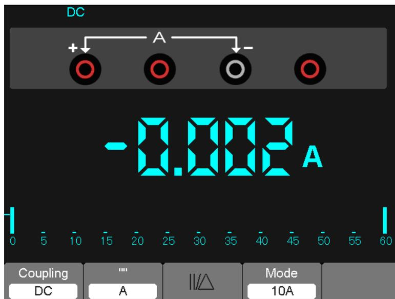
Figure 7-9 DC Current Measurement for 10A
