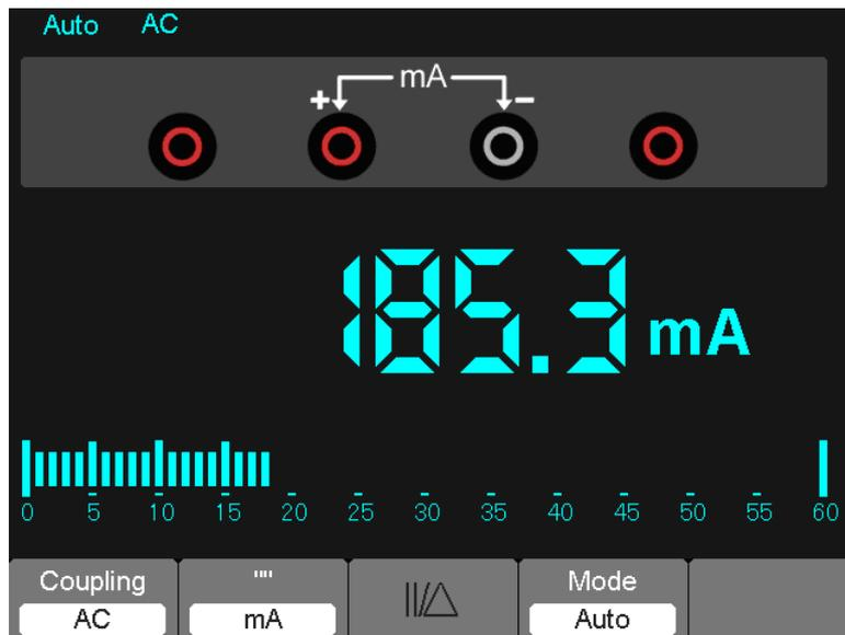
Figure 7-10 AC Current Measurement for 600 mA
