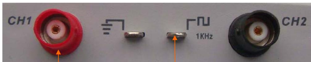
CH1: to connect with the probe
