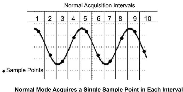
**Peak Detect:** Use this mode to detect glitches within 10ns and to limit the possibility of aliasing. This mode is valid at the TIME/DIV setting of 4 $\mu$ s/div or slower. Once you set the TIME/DIV setting to 4 $\mu$ s/div or faster, the acquisition mode will change to Normal because the sample rate is fast enough that Peak Detect is unnecessary. The oscilloscope does not display a message to tell you that the mode has been changed to Normal.
