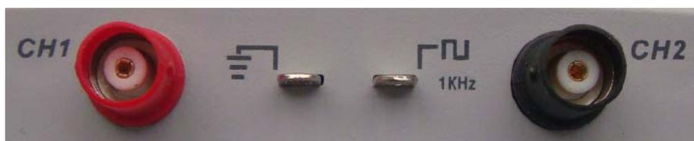
1. CH1, CH2: Input connectors for waveform display, through which to connect and input the signal to be measured.
