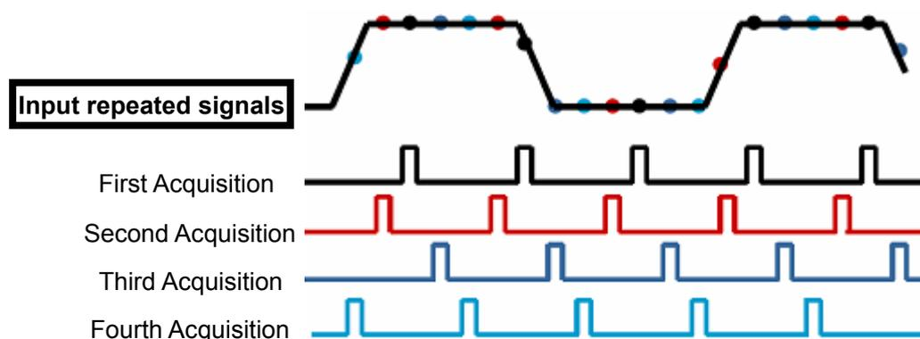
As shown above, acquire input signals (cycle repeatable) for more than once at a slow sample rate,
