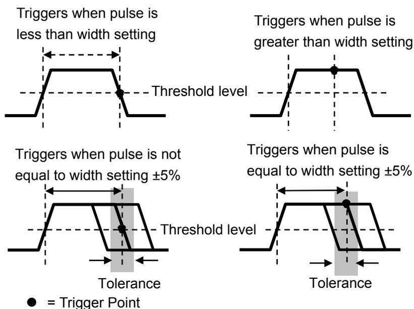
=, ≠: Within a  $\pm 5\%$  tolerance, triggers the oscilloscope when the signal pulse width is equal to or not equal to the specified pulse width.
