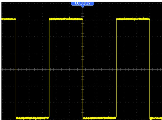
As shown in the above figure, you can get a stable waveform display if inputting a square wave at the frequency of 1KHz, with pulse width set to 500 $\mu$ s.
