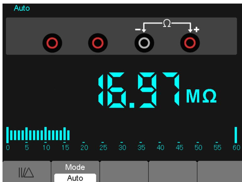
Figure 7-2 Resistance Measurement
