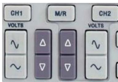
2. **Menu (CH1, CH2):** Display vertical menu options; turn on or off the display of channel waveforms.
