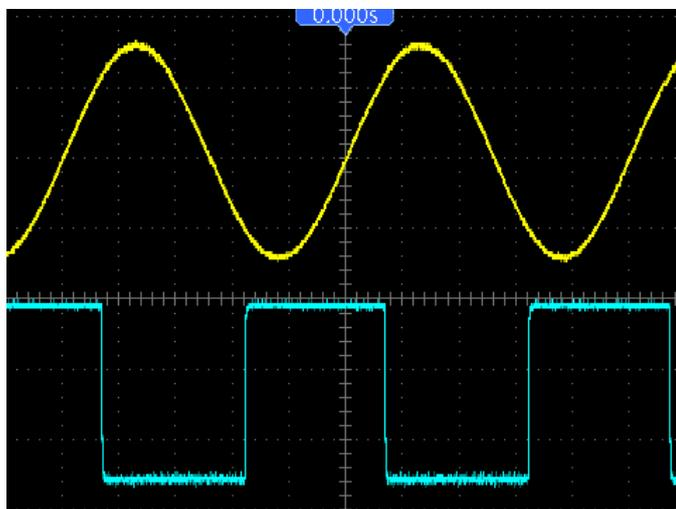
As illustrated in the above figure, input a 1KHz sine wave from CH1 and a 1KHz square wave from CH2.
