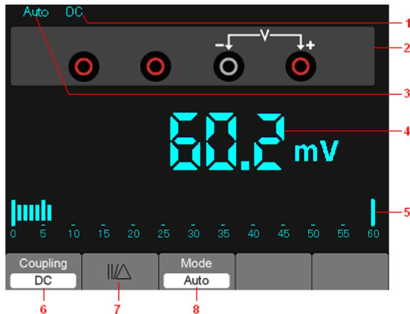
Figure 7-1 Multimeter operation window
