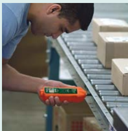
Accessory wheels enable tachometer to measure linear surface speeds
