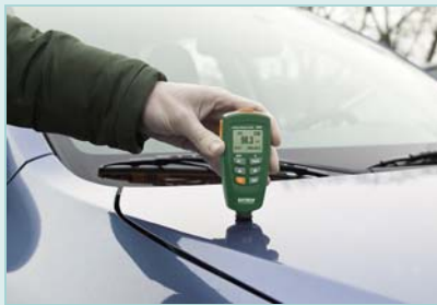
Measuring the thickness of automotive paint
